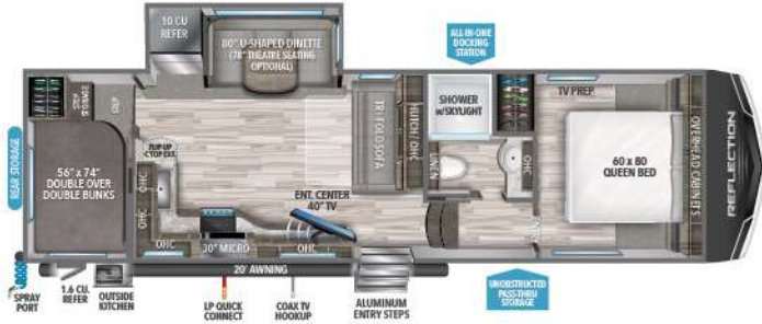
278BH UVW 1 8,345 HITCH 1 1,321 LENGTH 2 32' 11" HEIGHT 3 12' CAPACITY 56 78 39
