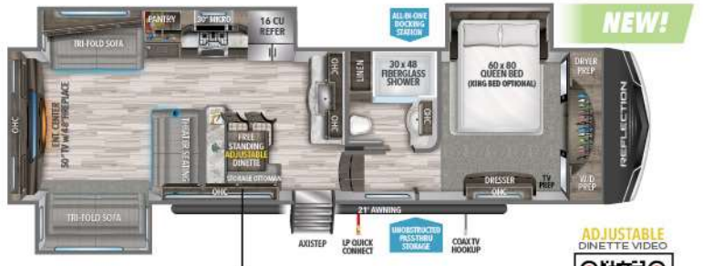
341RDS UVW 1 10,964 HITCH 1 2,072 LENGTH 2 36' 11" HEIGHT 3 12' 6" CAPACITY 74 87 47
