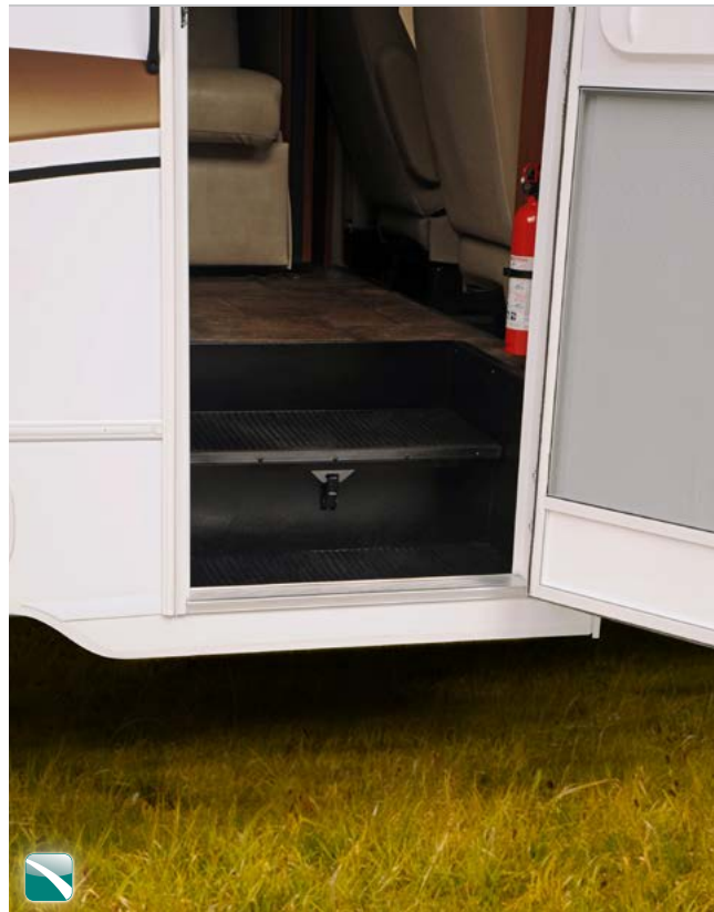
Lower Entrance Step is designed for easy access (Ford® Chassis) (Chevrolet® Chassis features a single pull-out step.)
